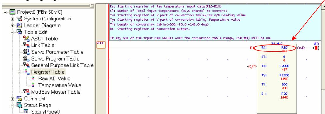
Description: The MLC (Multiple-segment Linear Conversion, FUN34) function instruction should be used to convert the raw reading value into the final temperature value when using this module, and also two register tables are necessary for proper operation with this instruction.
